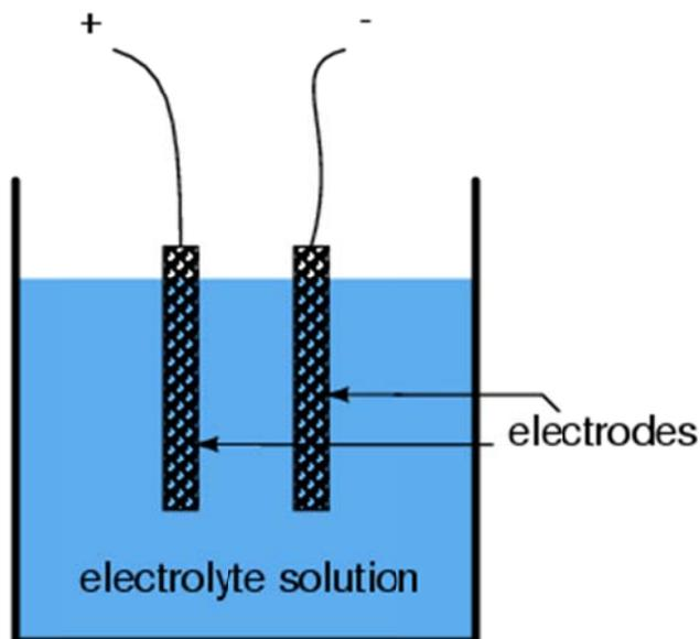
The two electrodes are made of different materials, both of which chemically react with the electrolyte in some form of ionic bonding.
