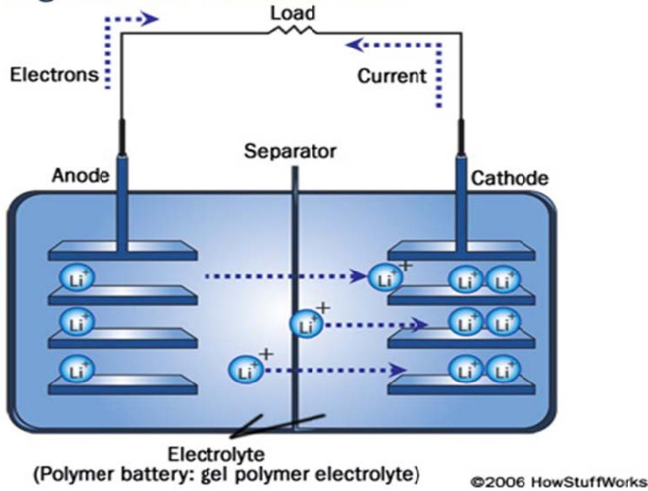
In order to engineer any battery to generate electricity one must have an anode and cathode composed of two different metals separated from each other bathed in an effective electrolyte. Include stripping of electrons, electrode collection of e-, role of metals, role of separator, role of electrolyte, what makes a good electrolyte, diagram of battery function with e- flow direction
