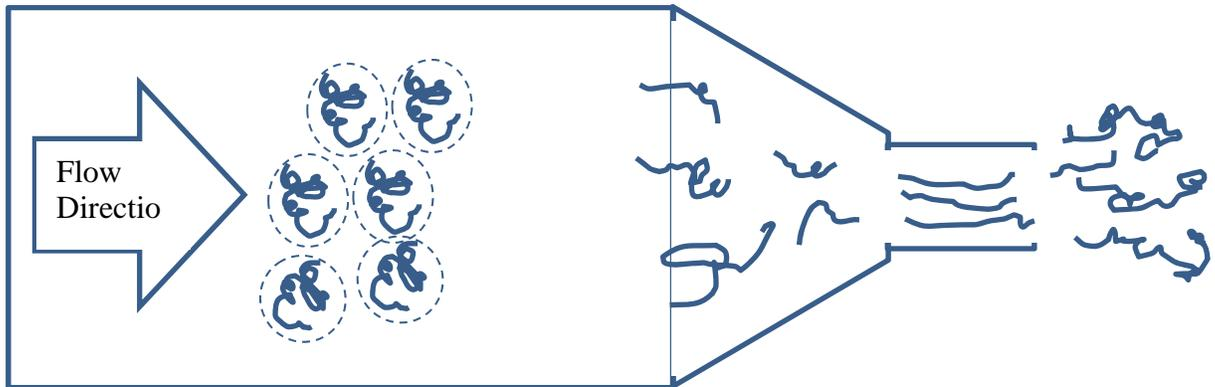
**Figure 1** In the large diameter section the polymer chains are relaxed and take up a more natural configuration. As the diameter restricts, the polymer chains get closer together and deviate from that equilibrium configuration. Once the polymers exit the die, it can return to a more favor shape by expanding.
