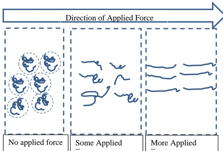
**Figure 2** When no force is applied, the polymer are in a relaxed state. As more and more force is applied (it is also depends on how quickly it is applied but we will save that for another day) the polymers stretch out and can slid past one another.
